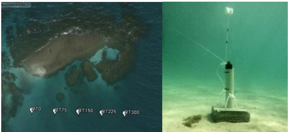
Figure 2: Positioning of the receivers near Ilha da Barra reef during the range tests (left) and mooring used to place the receivers (right), with two transmitters over it.
